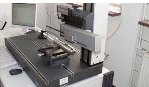
Pomiar zarysu i kontrola optyczna Measurement of outline and optical inspection
